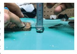
feeler gauge and measure the gap between the bottom of the string and the top of the eighth fret (measuring from fret wire itself, not the fingerboard), which is where the curvature should be deepest.
