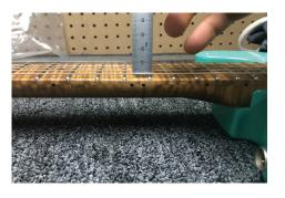
increments of .010" (ten thousandths of an inch). When the bottom of a mark aligns with the bottom of the string, that measurement is the string height at that point. Note: Each marking on the gauge is .005" thick. This is why string scale measurements are in .005" increments. **To adjust saddle**
